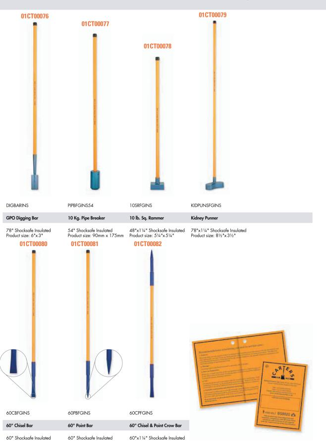
BS8020:2002 is an exacting specification that demands full adherence to detailed manufacturing and testing procedures for safe working practices to be maintained by the user when working on or in close proximity to live conductor cables. Every single tool is flash tested to 10,000 Volts before the issue of a certificate, unique to each implement. Our guarantee of safety to the user, in a potentially dangerous live-working environment.
